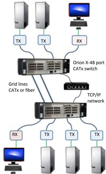
Structure of a matrix grid network
