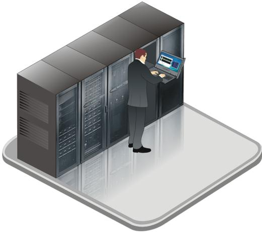
**Installation** RackView Sideways 24" is very easy to install. Simply adjust the rack-rail length to the depth of your rack, slide the unit through the rack, and secure the rack mount brackets to the front and rear rack rails with the supplied 8x M6 screws, cage nuts, and cup washers. A cable is supplied that connects the video, keyboard, and mouse signals to your host computer DVI or HDMI and USB.
